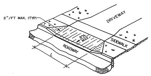
NOTE: THE L DISTANCE SHOULD BE ADEQUATE TO ACCOMMODATE TURNING VEHICLES.
